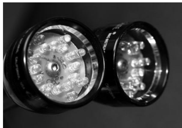
FIG. 2—Ultraviolet-light-emitting-diode “forensic flashlights.” These particular units are modified, commercially available standard flashlights that operate on 3 “C” batteries.
