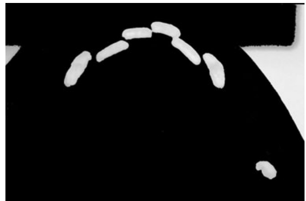
FIG. 5—Cropped portion of Fig. 5 with "Otsu Thresholding (Region 2)" filter plug-in applied via the ImageJ software program.
