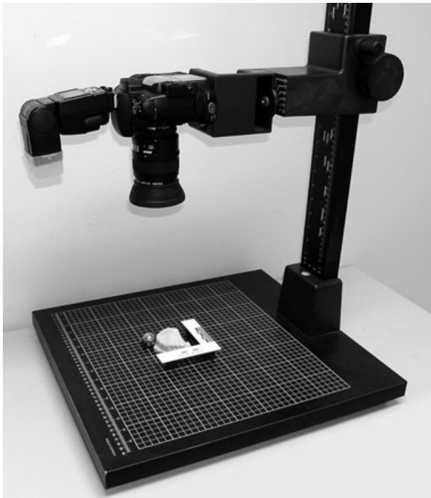
FIG. 3—Photographic copy stand. (The camera's flash unit is not used in this technique.)
